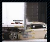
that passenger vehicles will be prevented from the underride hazard. Strengthening can be achieved with additional supports, diagonal braces and gusset plates. US trailers are now slowly adopting side guards, mostly for aerodynamic fuel-efficiency reasons, and they, too, must be made much stronger.
