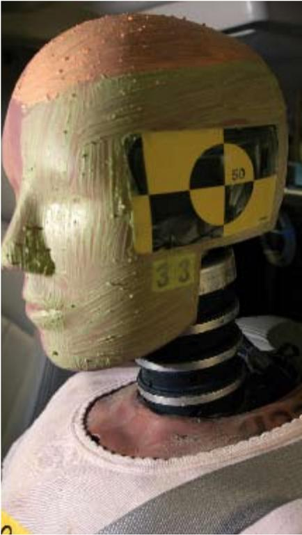
Above: A crash dummy sits in a 2006 Buick Rainier at GM's rollover crash testing facility. The US\$10 million facility will be used to study ways to reduce injuries and deaths in rollover crashes by developing sensors for air bags that can help protect occupants in a rollover and help keep them from being ejected from the vehicle
