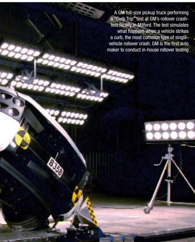
A GM full-size pickup truck performing a "Curb Trip" test at GM's rollover crash-test facility in Milford. The test simulates what happens when a vehicle strikes a curb, the most common type of single-vehicle rollover crash. GM is the first auto maker to conduct in-house rollover testing
