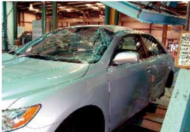
This Toyota Camry had "full load" applied, which means 4.3 times the vehicle weight, therefore a strength-to-weight ratio (SWR) of 4.3, well above the level of 2.5 to three that the NHTSA is currently considering
